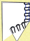
Figure 8 Stitches should hang over the edge a little to create a flat seam when fabrics are pulled apart.
